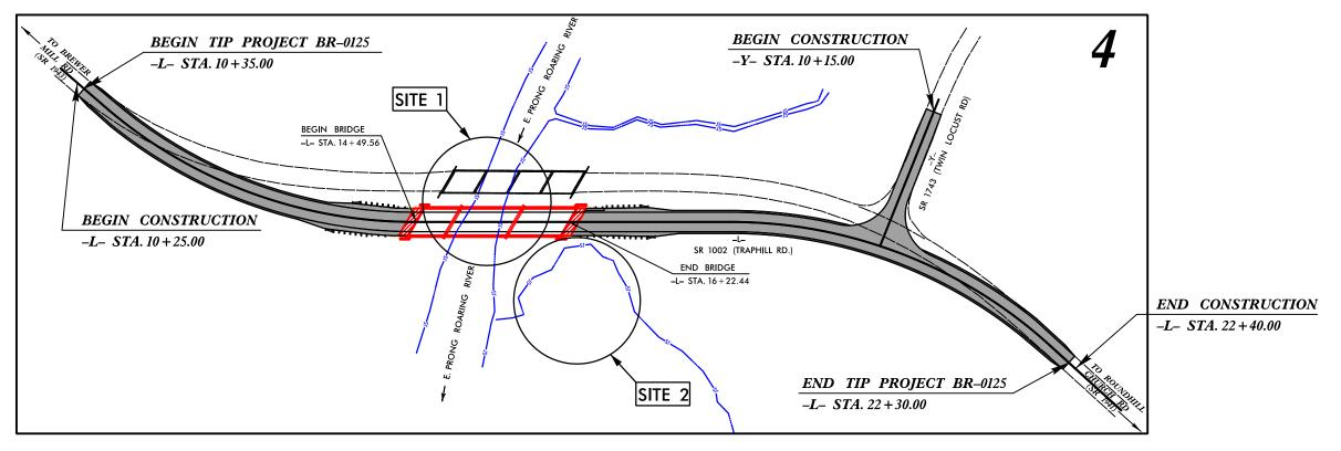
DESIGN EXCEPTION REQUIRED FOR HORIZONTAL CURVE RADIUS AND VERTICAL CURVE K-VALUE & NIGHTTIME SSD. THIS PROJECT IS NOT WITHIN ANY MUNICIPAL BOUNDARIES. CLEARING ON THIS PROJECT SHALL BE PERFORMED TO THE LIMITS ESTABLISHED BY METHOD
