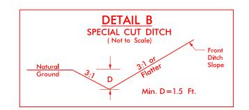
FROM STA. 23+35 TO STA. 24+10 -L- LT FROM STA. 24+90 TO STA. 27+00 -L- LT
