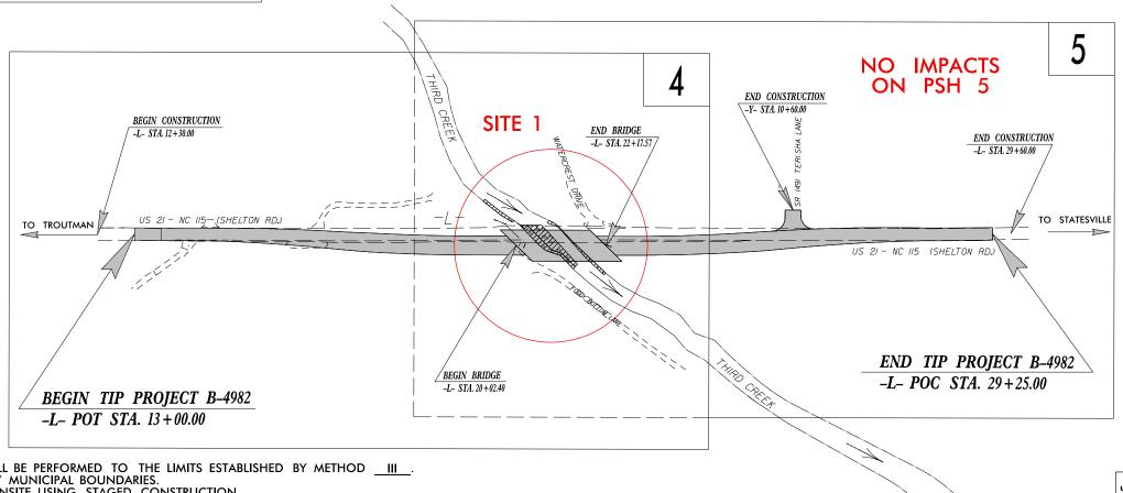
CLEARING ON THIS PROJECT SHALL BE PERFORMED TO THE LIMITS ESTABLISHED BY METHOD III . THIS PROJECT IS NOT WITHIN ANY MUNICIPAL BOUNDARIES. TRAFFIC IS TO BE MAINTAINED ONSITE USING STAGED CONSTRUCTION.
