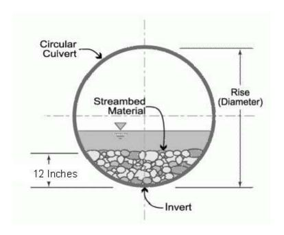
In all other counties: Culverts greater than 48 inches in diameter will be buried at least one foot below the bed of the stream. Culverts 48 inches in diameter or less shall be buried or placed on the stream bed as practicable and appropriate to maintain aquatic passage, and every effort shall be made to maintain the existing channel slope. The bottom of the culvert must be placed at a
