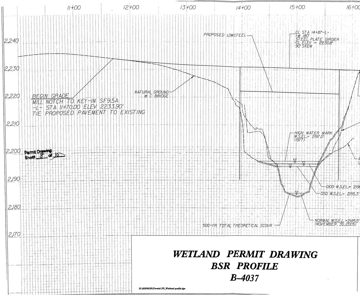
16+00 SCALE |" = 50' H |" = 10' V END GRADE -L- STA 16+13.75 = -Y/- STA 10+98.00 (9' RT) ELEV 2230.06 -1 - 57A 16 + 22.75 =-YI- STA 10+98.00 ELEV 2230.24' ¢ LOW POINT NATURAL GROUND DOWNSTREAM NATURAL GROUND UPSTREAM -0100-W.S.EL.= 2196.1' **NCDOT DIVISION OF HIGHWAYS BUNCOMBE COUNTY PROJECT:** 33403.1.1 (B-4037) **REPLACEMENT OF BRIDGE NO.262** OVER SOUTH HOMINY CREEK ON SR 3452 0/12/2007
