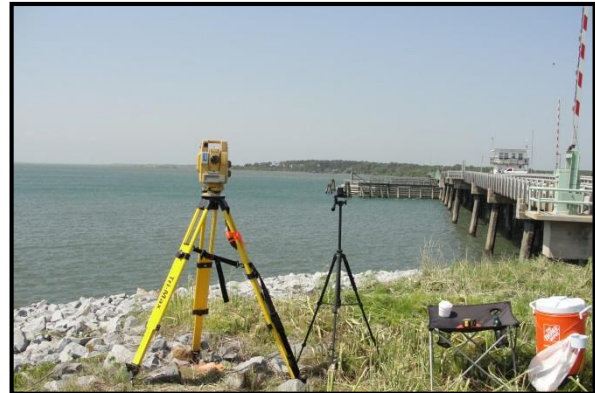
Survey equipment set up on southwest side of Harkers Island Bridge
