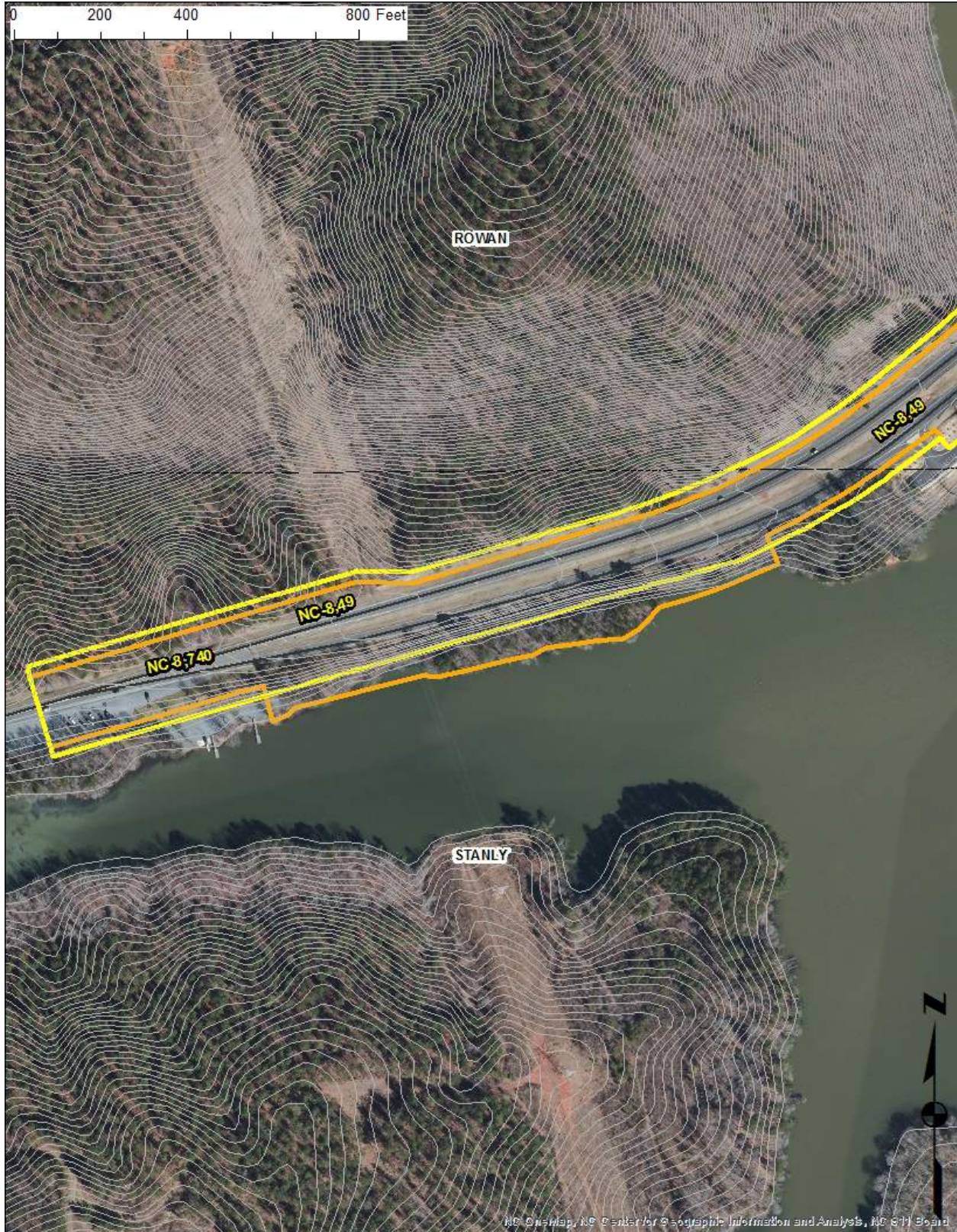
Aerial photograph with 2-foot contours illustrating the western end of the proposed project, the original APE (yellow) and the updated APE (orange) accommodating temporary water access.
