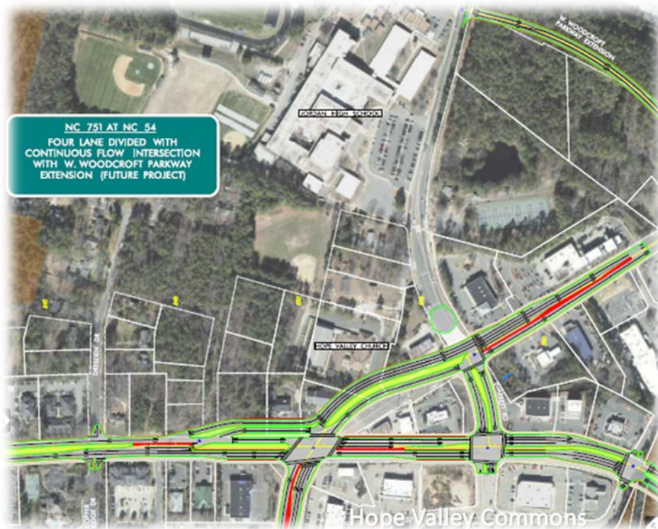
Figure 26. NC 751/Garrett Road continuous flow intersection option
