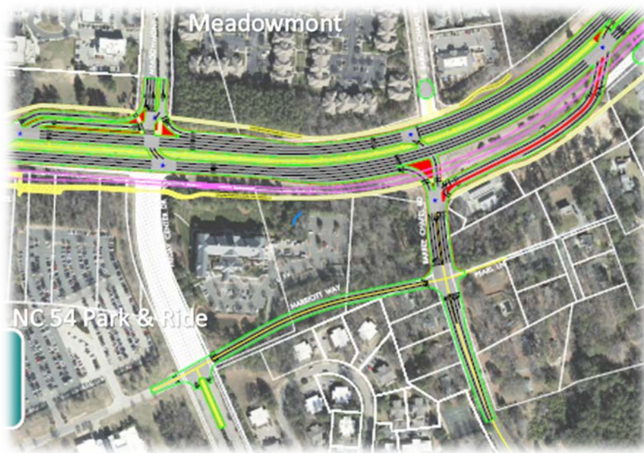
Figure 15. Offset Continuous Flow Intersection Option
