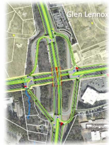
Figure 6. US 15/501 interchange half partial cloverleaf/half synchronized street option
