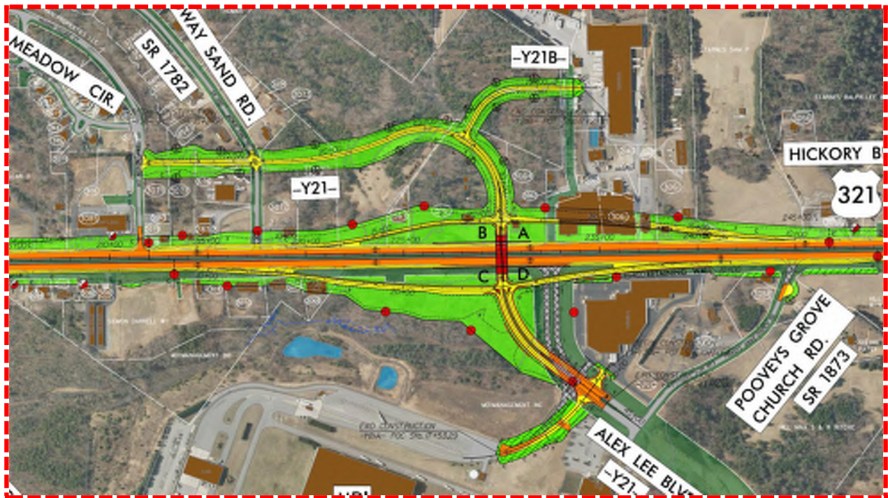
Figure 10: (Recommended) Tight diamond interchange design
