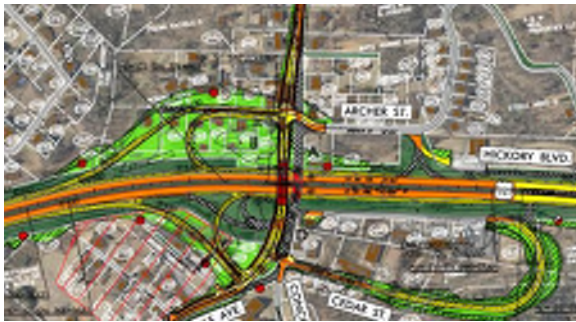
Figure 11: Partial cloverleaf interchange design
