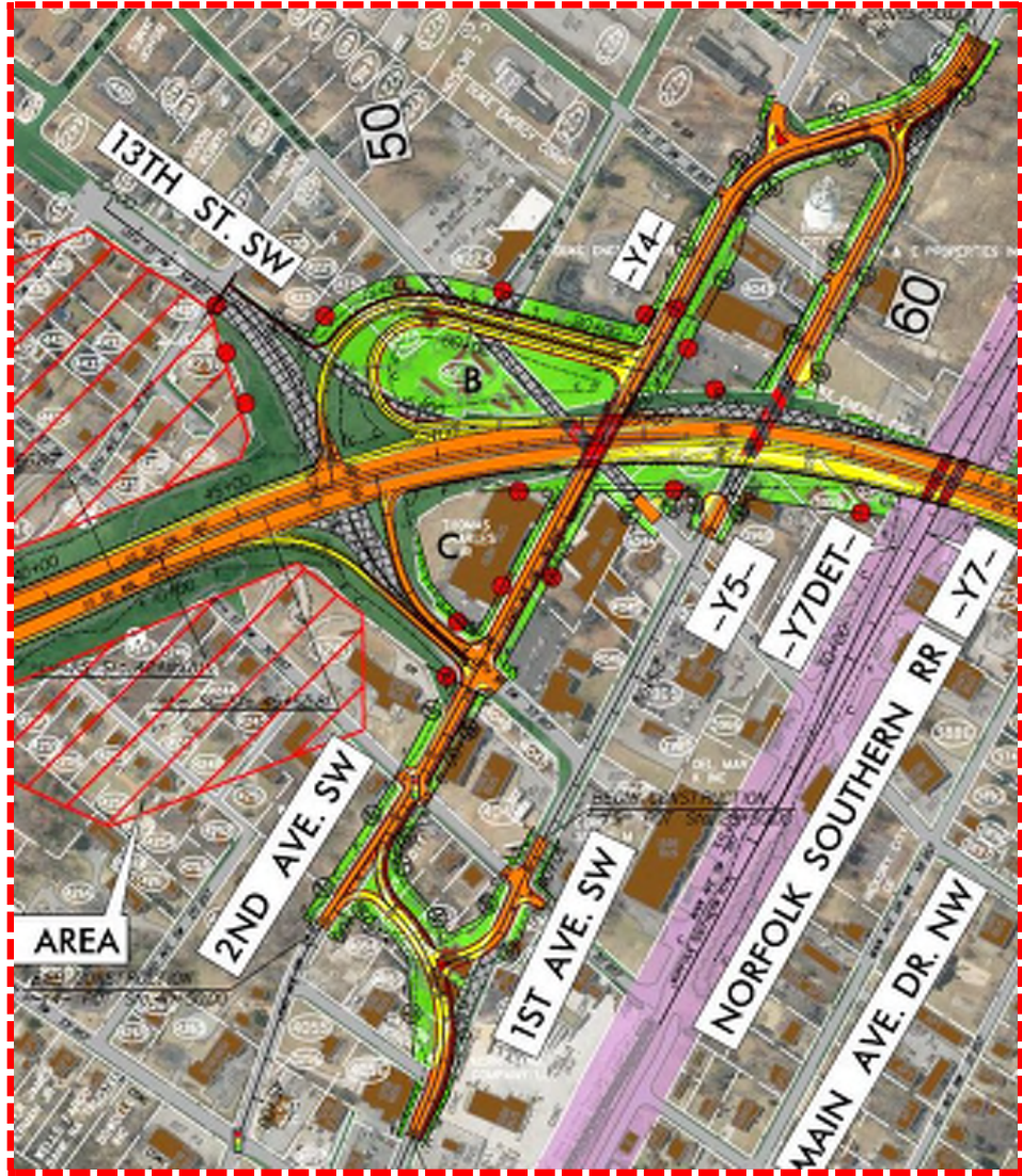
Figure 2: (Recommended) 2nd Avenue SW interchange design
