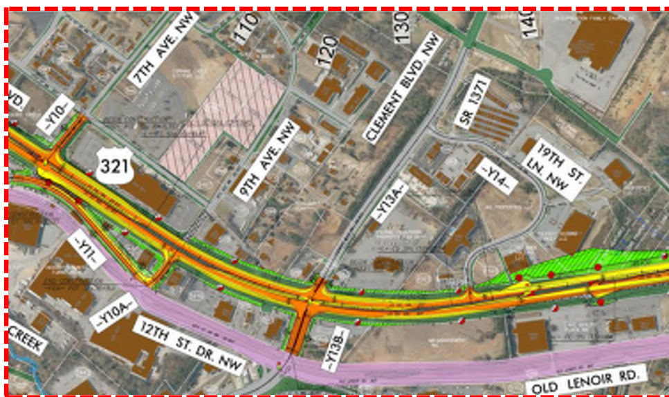
Figure 4: (Recommended) Superstreet intersection design
