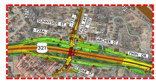
Figure 19: (Recommended)Tight diamond interchange design, January 2018
