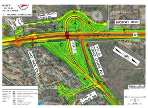
Figure 6: Trumpet interchange design, July 2016 public hearing (plus Wolfe Rd connector)
