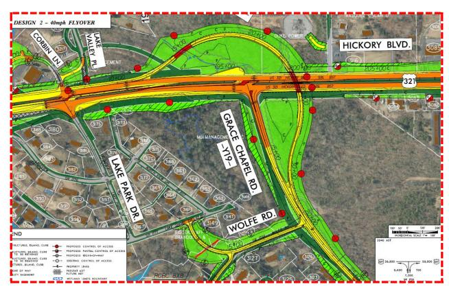
Figure 11: (Recommended) Revised flyover design, October 2017 public meeting with additional bridge over stream and increased slopes
