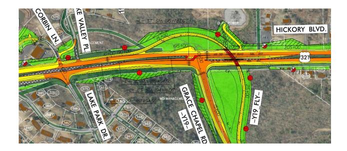
Trumpet Interchange (shown at the July 2016 public hearing) — This interchange would provide direct connection between US 321 and Grace Chapel Road. A new road would connect Lake Valley Place and the power station.
