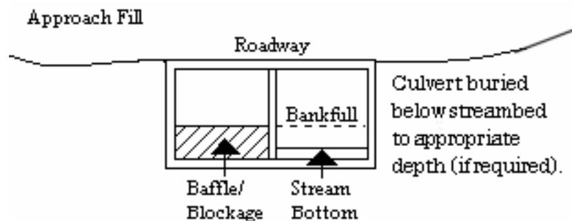
**3.6.3** Where adjacent floodplain is available, flows exceeding bank-full should be accommodated by installing culverts at the floodplain elevation. Additional culverts or culvert barrels at such crossings should not be buried, or if buried, must have sills at the inlets to ensure that they only receive flows exceeding bank-full.
