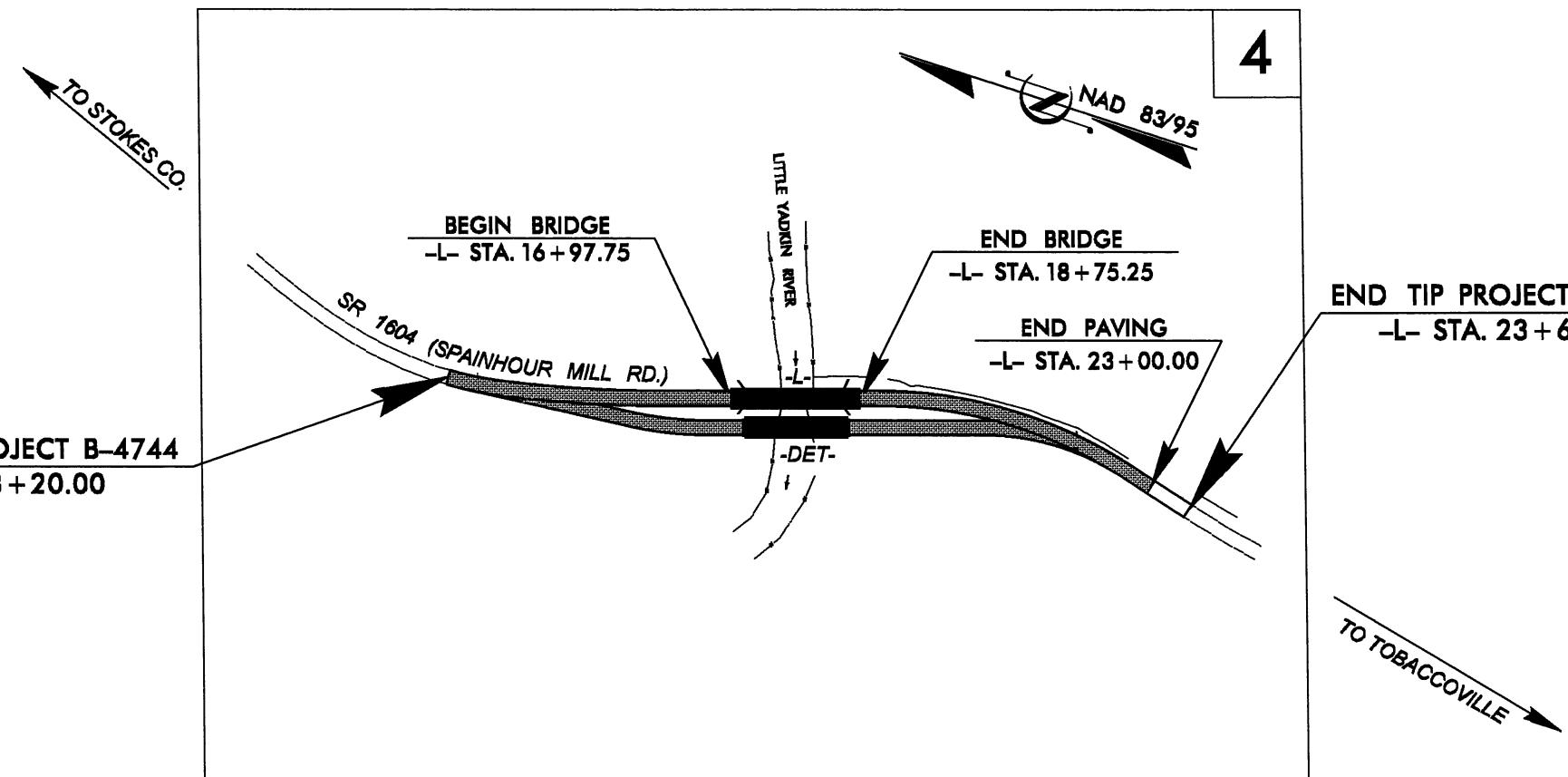
DESIGN EXCEPTION REQUIRED FOR SAG VERTICAL CURVE K-VALUES AND ASSOCIATED NIGHTTIME SSD CLEARING ON THIS PROJECT SHALL BE PERFORMED TO THE LIMITS ESTABLISHED BY METHOD III.
