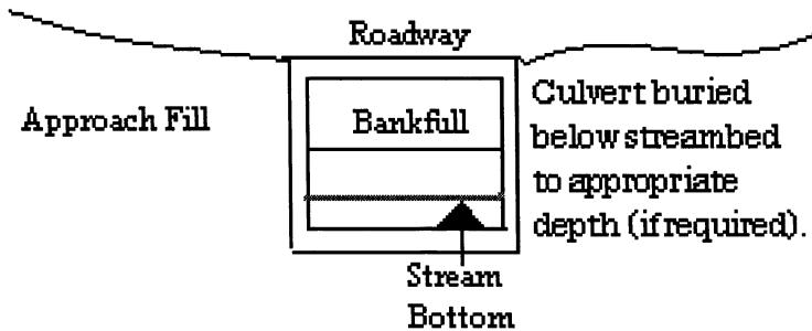
In all other counties: Culverts greater than 48 inches in diameter will be buried at least one foot below the bed of the stream. Culverts 48 inches in diameter or less shall be buried or placed on the stream bed as practicable and appropriate to maintain aquatic passage, and every effort shall be made to maintain the existing channel slope. The bottom of the culvert must be placed at a depth below the natural stream bottom to provide for passage during drought or low flow conditions.
