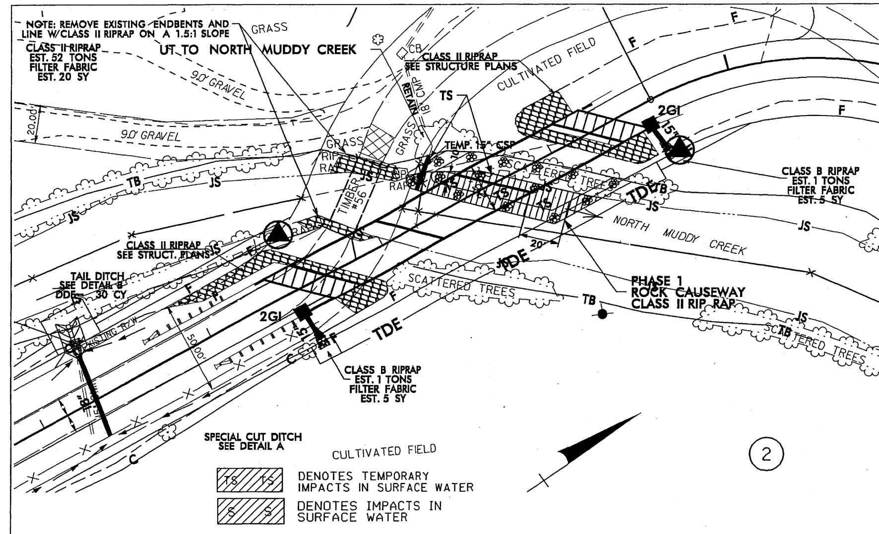
INSTALL ROCK CAUSEWAY AT BENT #2 AND CONSTRUCT BENT. REMOVE ROCK CAUSEWAY.
