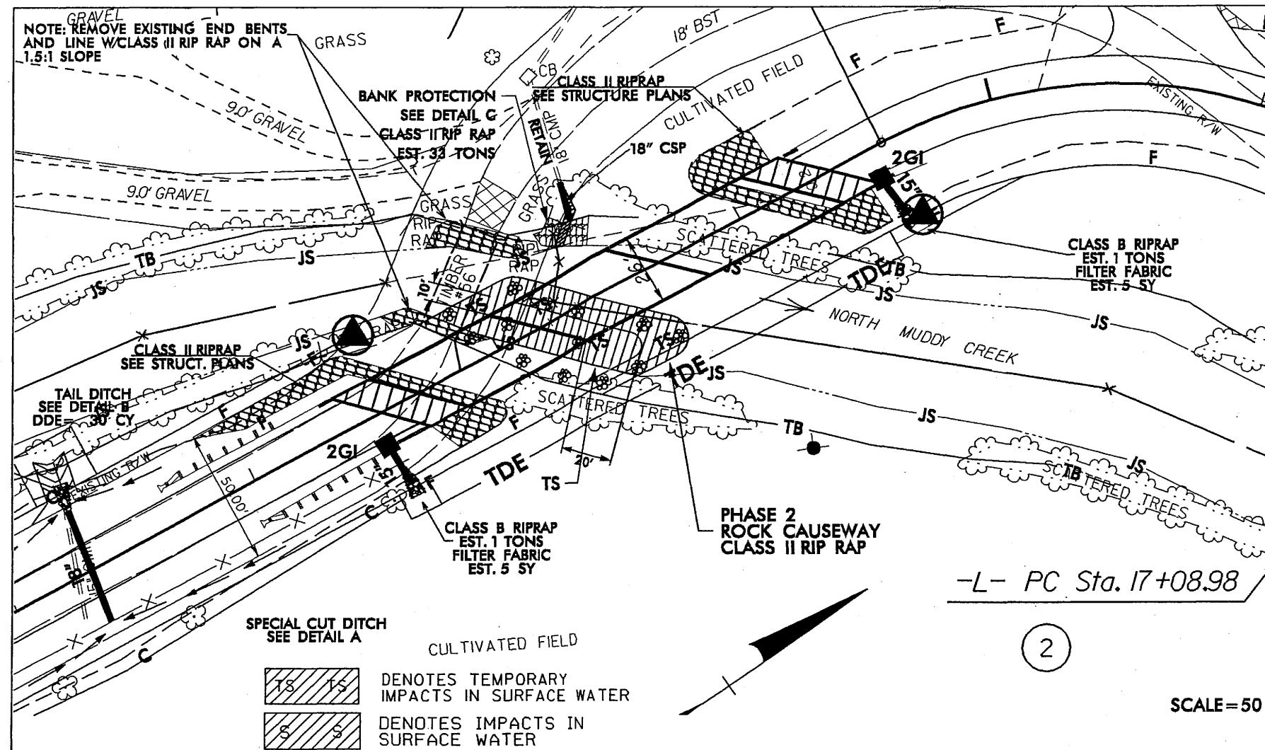
**INSTALL ROCK CAUSEWAY AT BENT #1 AND CONSTRUCT BENT. USE ROCK CAUSEWAY TO SET GIRDERS. REMOVE ROCK CAUSEWAY.**
