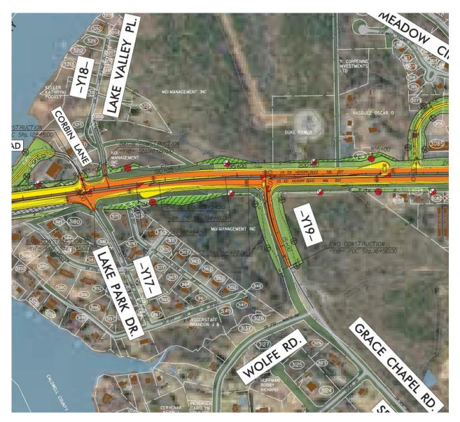
Flyover with a Superstreet Intersection (modified October 2017) – An elevated road would provide a direct connection from Grace Chapel Road to southbound US 321. All other movements will be controlled with an at-grade signalized intersection. Modification from the Flyover with a Superstreet Intersection Alternative design originally shown in 2016 includes adding a new connector from Lake Shore Drive to Grace Chapel Road via Wolfe Road.
