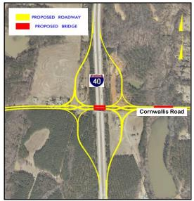
(B) New Interchange at Cornwallis Road (SR 1525) A DDI is proposed at the existing Cornwallis grade separation. Improvements also include widening Cornwallis Road from NC 50 to just east of Shiloh Road and reconfiguring the intersection of Cornwallis Road with NC 50 (Old Drugstore Road).
