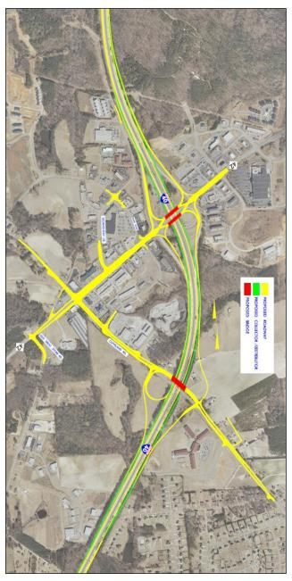
(C) New Collector-Distributor System and Diamond Interchange at Cleveland Road (SR 1010)
