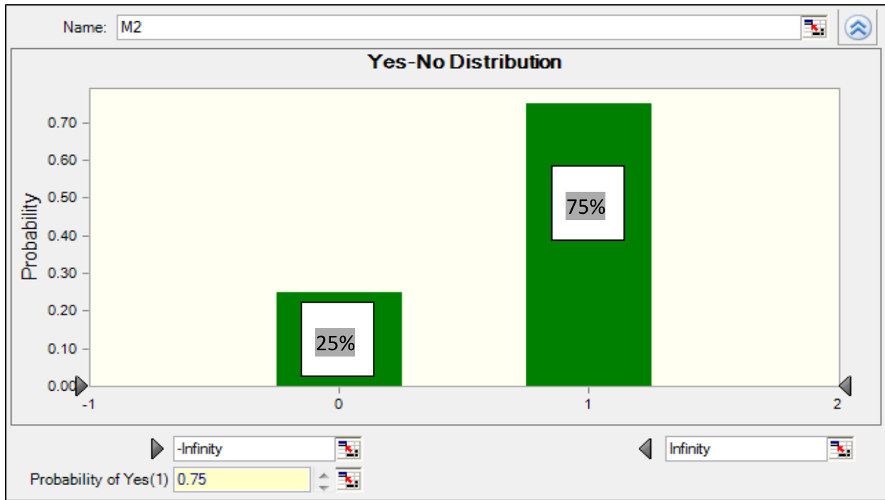
Figure 5 - Example of Binomial Distribution for a Project Risk's Likelihood of Occurrence
