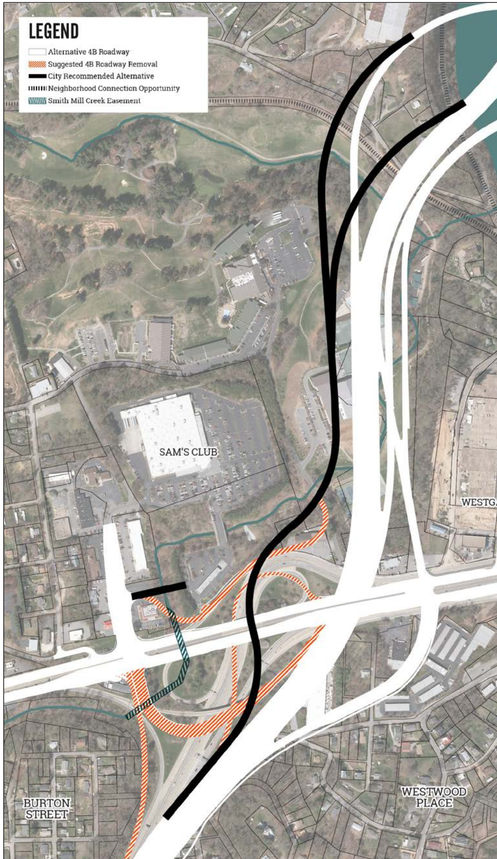
Figure 9: Conceptual drawing of SB I-26 ramps with Patton Avenue with alternative (black) ramps that could replace the original Alternative 4-b alignment (orange) and the remaining NCDOT proposed alignment (white)
