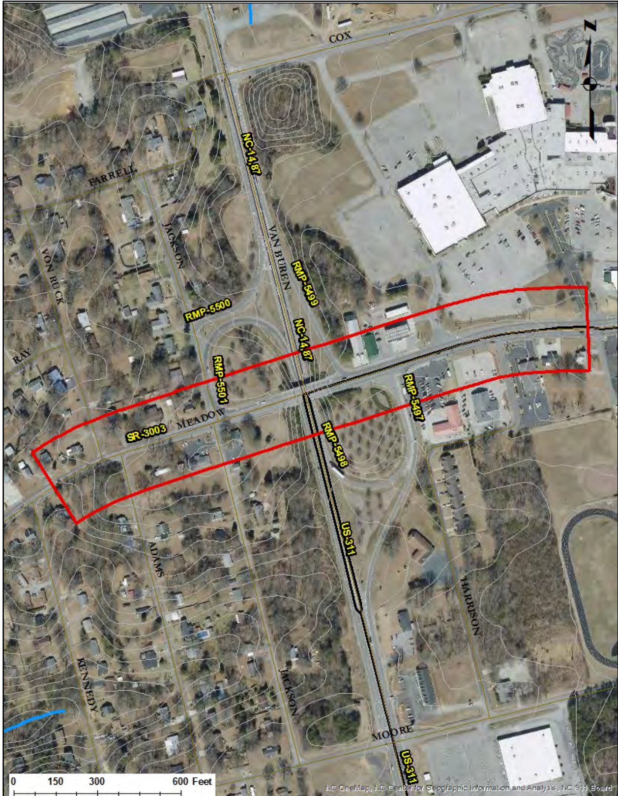
Aerial photograph with 2-foot contours illustrating the location of the proposed APE (red lines) for the replacement of Bridge No. 108 on US 311/NC 700.
