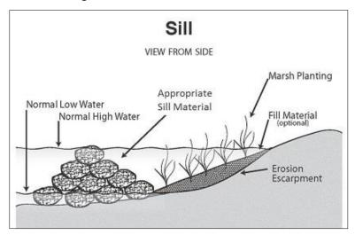
Figure 8. Schematic of a living shoreline that includes a sill feature. Drawing by NCDEQ, no date.
