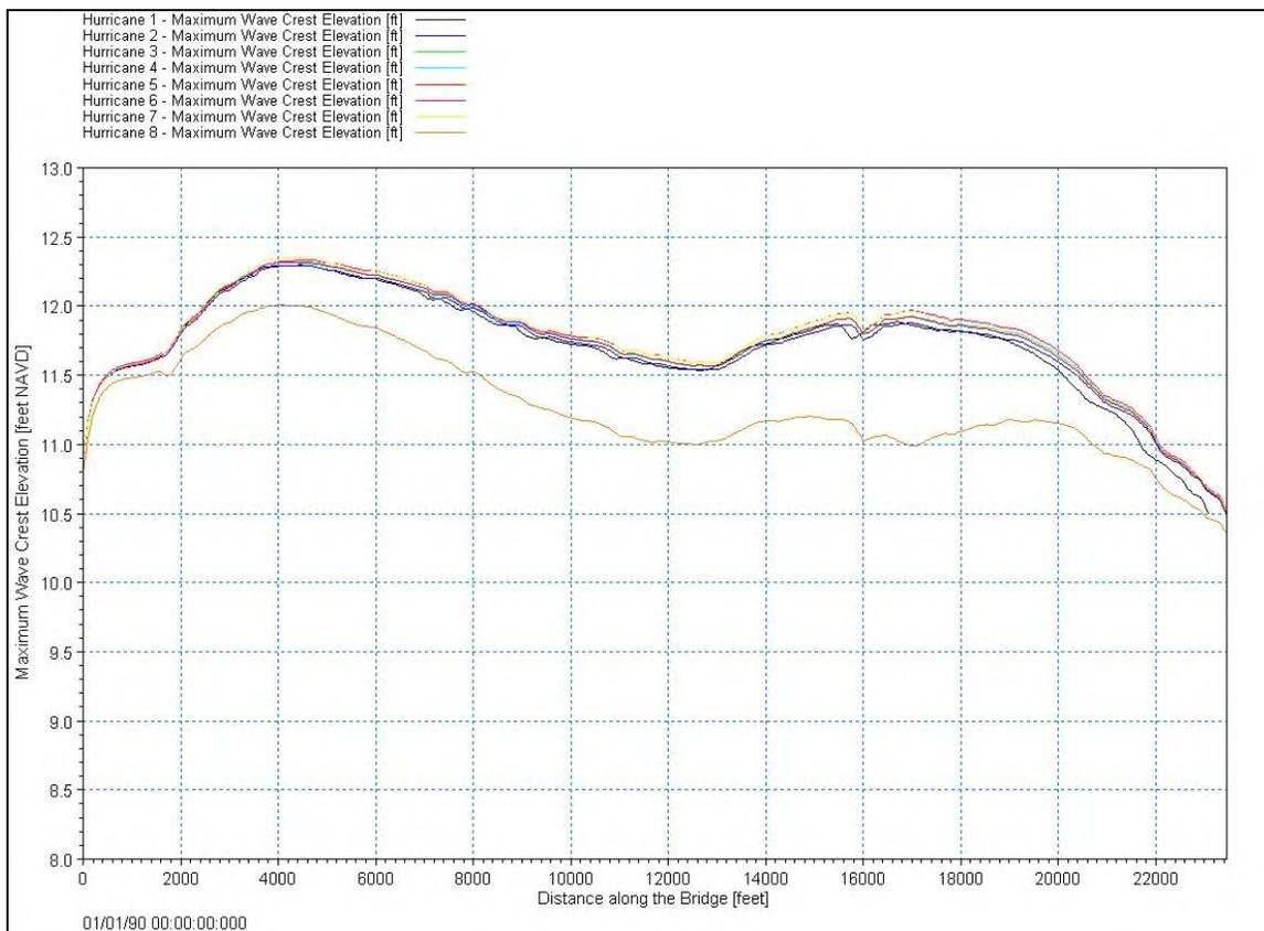
**Figure 5.16: Maximum Wave Crest Elevation along the Proposed Bridge Location**
