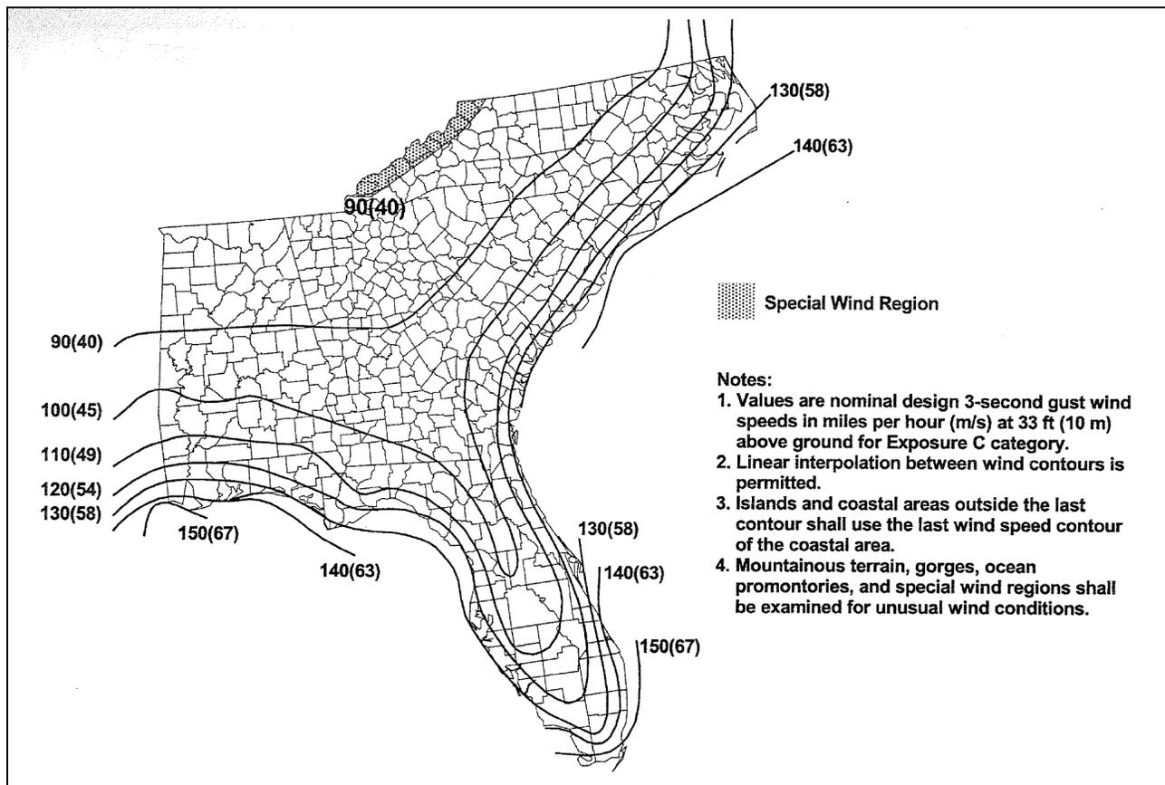
**Figure 5.2: Basic Wind Speed – Eastern Gulf of Mexico and South-eastern US
