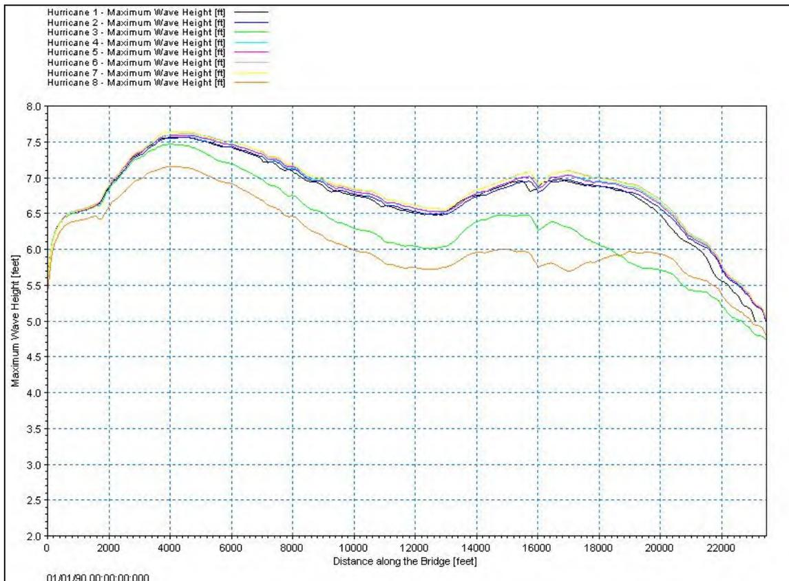
**Figure 5.15: Maximum Wave Height along the Proposed Bridge Location**
