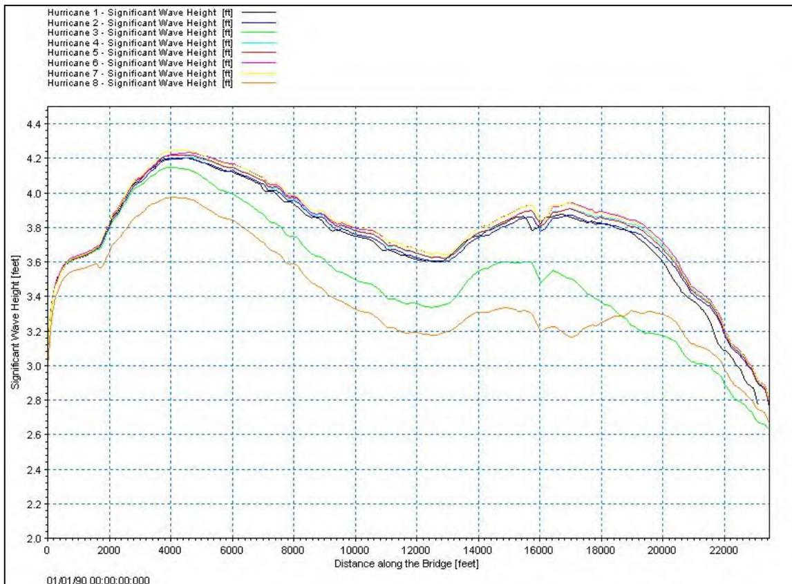
**Figure 5.13: Maximum Significant Wave Height along the Proposed Bridge Location**
