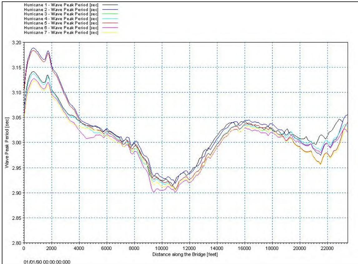
**Figure 5.14: Maximum Wave Peak Period along the Proposed Bridge Location**
