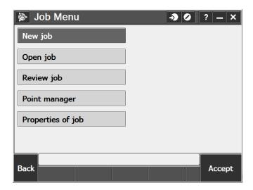
After pressing 'New Job' the following screen is displayed. The difference between creating an EDM calibration job and a typical NCDOT Trimble job is that distance units must be set to Meters. All the other settings can be set as usual. Press 'Accept' to create the job, and return to the main screen.
