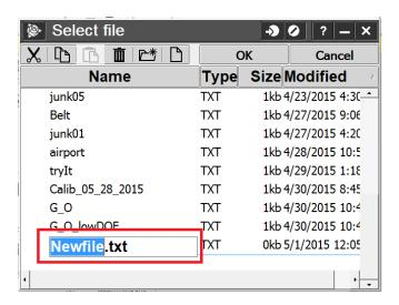
After creating the file, the name of the new file is displayed in the following screen, and a new 'Details' button is now displayed. Two new soft key options, 'Process' and 'Measure, are now displayed when both the published EDM baseline and the measured EDM baseline file have been defined. Though the 'Process' button is displayed choosing it with a new file would generate a warning message since no measurements have been collected. Press the 'Details' button.
