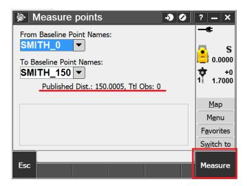
After the distance measurement has been collected the following screen is displayed allowing the review of the measurement before storing the measurement to the file. It's a good idea to compare the published distance to the measured horizontal distance before storing the measurement. Typically, there should only be a few millimeters difference between the measured and the published distance. Press the 'Store' soft key after reviewing the measurement.
