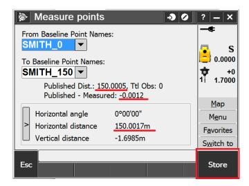
After an observation has been stored the 'Process' button is available if three or more distances have been collected. Press the soft key 'Process' to obtain the results of the calibration.
