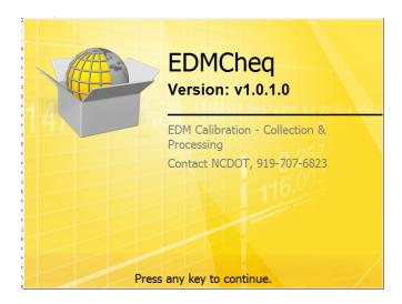
Following is the opening screen of the EDM calibration program. A new job should be created for every calibration performed.
