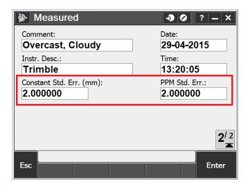
After defining the published EDM baseline and creating the measured EDM baseline file the next step is to collect the horizontal distance measurements. Press the 'Measure' soft key to begin the data collection procedure.
