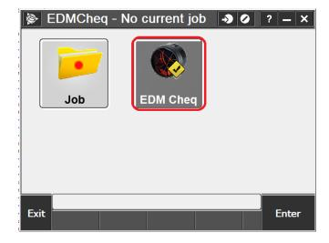
The collection, processing, editing and reviewing of the EDM calibration is initiated from the following screen. First, the published EDM baseline being used has to be designated. Press the 'Define Published EDM BL' button.
