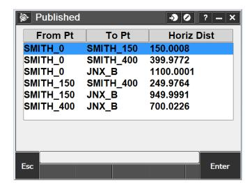
After the published baseline has been chosen a new data file containing the measured horizontal distances needs to be created if a new calibration is being performed. An existing measurement calibration file can also be opened for review, editing, reprocessing, and appending. Press the 'Define Measured EDM BL' button to create a new measurement file or open an existing measurement file.
