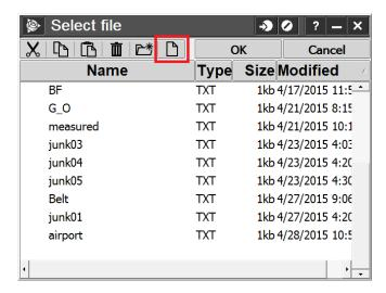
Enter the name of the new file. This file is an ASCII file containing the station names and horizontal distance measurements.
