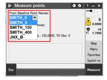
The published distance is displayed as well as the total number of observations that have been collected. Make sure you are leveled and sighting the 'To' point then Press the 'Measure' soft key to initiate the measurement.
