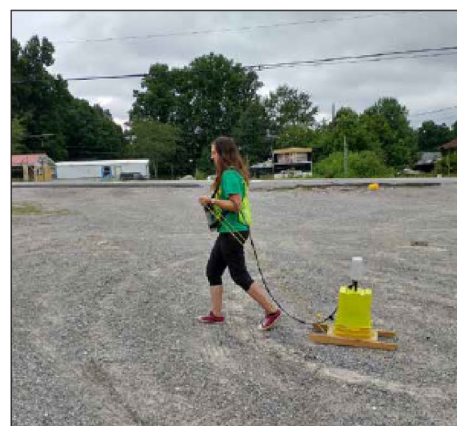
Photo 3. Collecting magnetometer data at Parcel #025.
