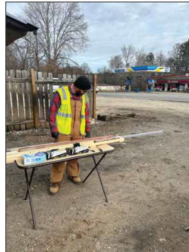
Photo 5. Describing soil cores.
