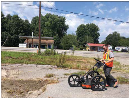
Photo 1. Collecting GPR data at Parcel #014.
