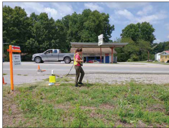
Photo 2. Collecting magnetometer data at Parcel #014.
