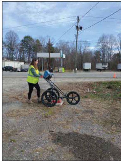
Photo 1. Collecting GPR data in Grid 1.
