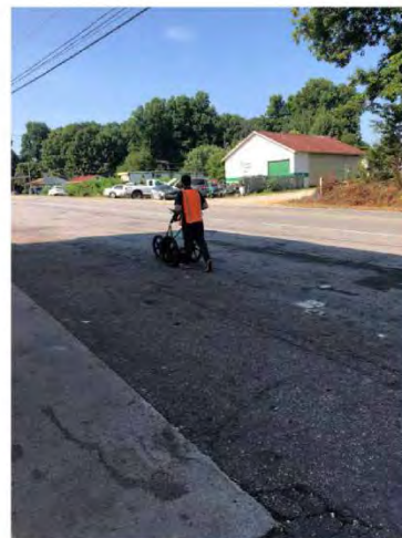
Photo 3. Using the GPR to clear locations for potential borings
