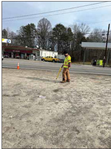
Photo 2. Checking Grid 1 for magnetic anomalies with the Schonstedt.
