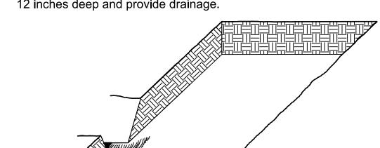
3. Backfill the trench with 2 inches well rotted sawdust. Place a 2 inch layer of well rotted sawdust at a sloping angle at one end of the trench.
