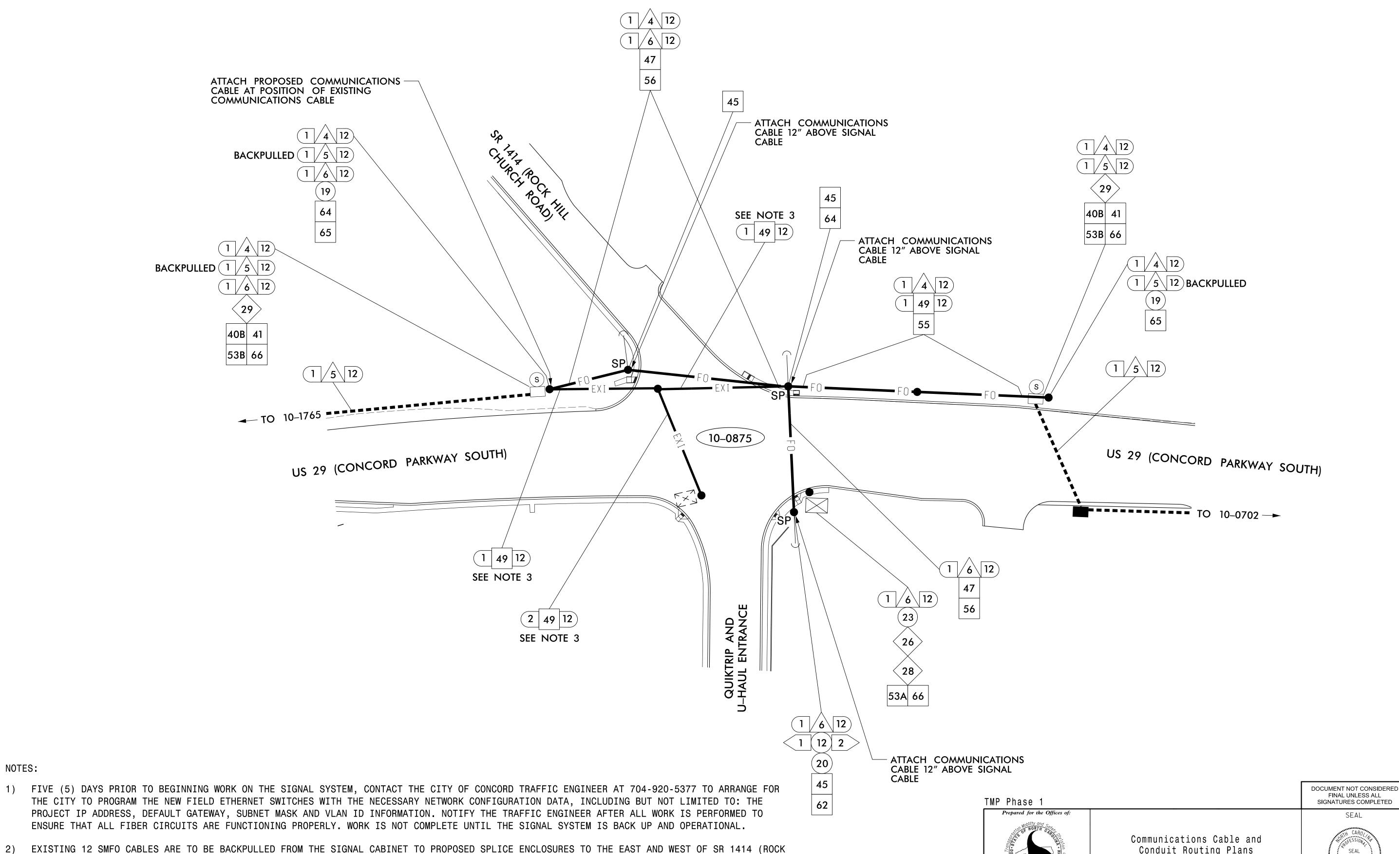
REMOVE EXISTING MESSENGER CABLE AFTER BACKPULLING COMMUNICATIONS CABLES TO NEW SPLICE ENCLOSURES.
