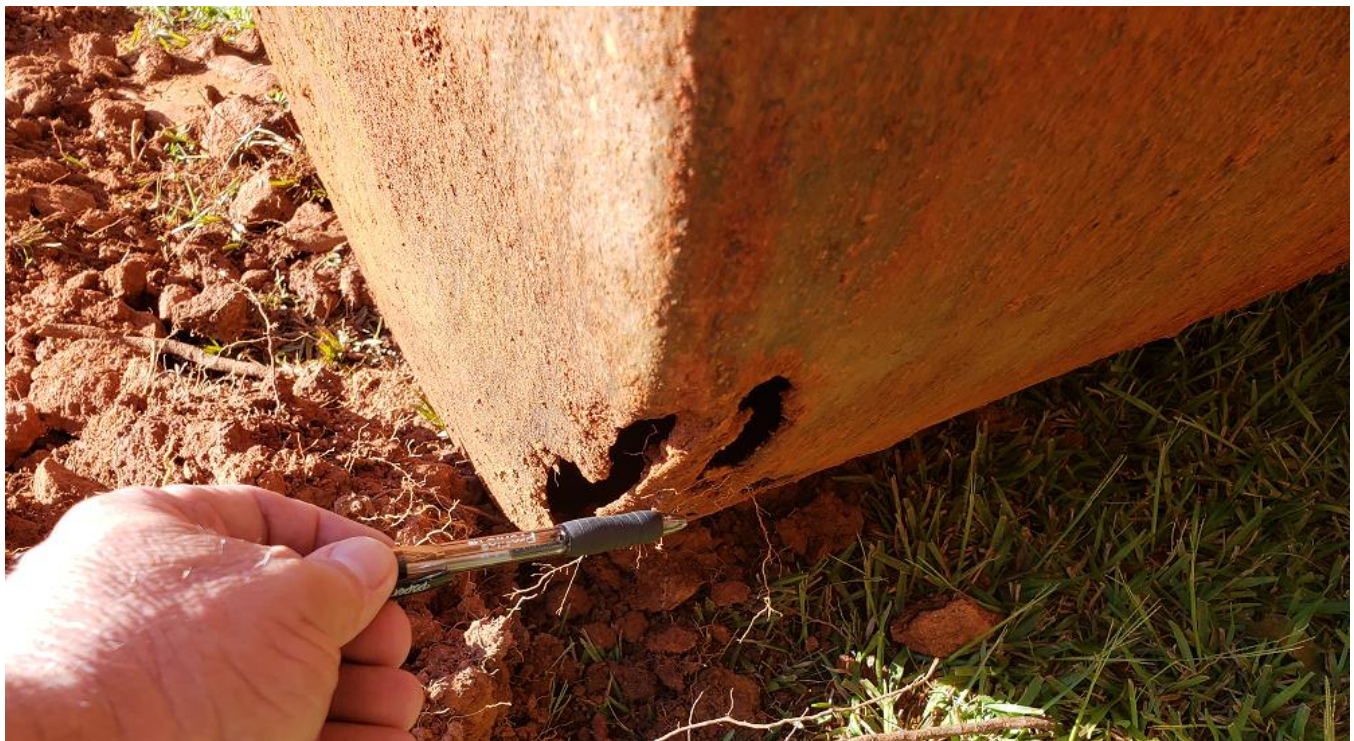
Photograph 8: Holes Observed in UST
