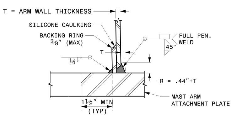
SECTION B-B FULL-PENETRATION GROOVE WELD DETAIL
