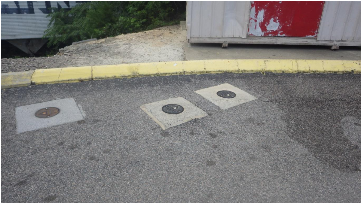
Clustered monitoring wells (Type III and Type II)
