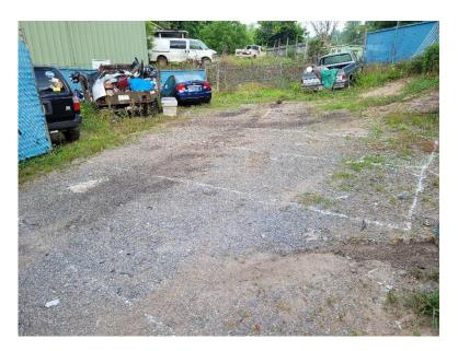
UST basin area in the northern portion of the site with apparent surface staining. Soil Borings 1-4 advanced around all sides of the UST basin area.
