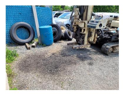
Apparent surface staining in front of the northern bay door. Location of Soil Boring 6.
