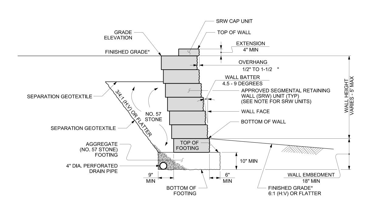
A FENCE OR HANDRAIL IS REQUIRED ON THE TOP OF RETAINING WALL NO. 1 AND 2. SEE ROADWAY PLANS FOR FENCE OR HANDRAIL ATTACHMENT DETAILS. DO NOT ATTACH FENCES OR HANDRAILS TO STANDARD SEGMENTAL GRAVITY WALLS.
