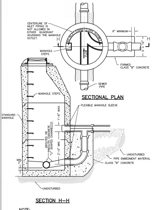
1. DROP CONNECTION IS NOT PERMITTED FOR HIGH VELOCITY SEWER MAINS MAINTAIN MINIMUM OF 8" OF CLEARANCE BETWEEN DROP CONNECTION AND
