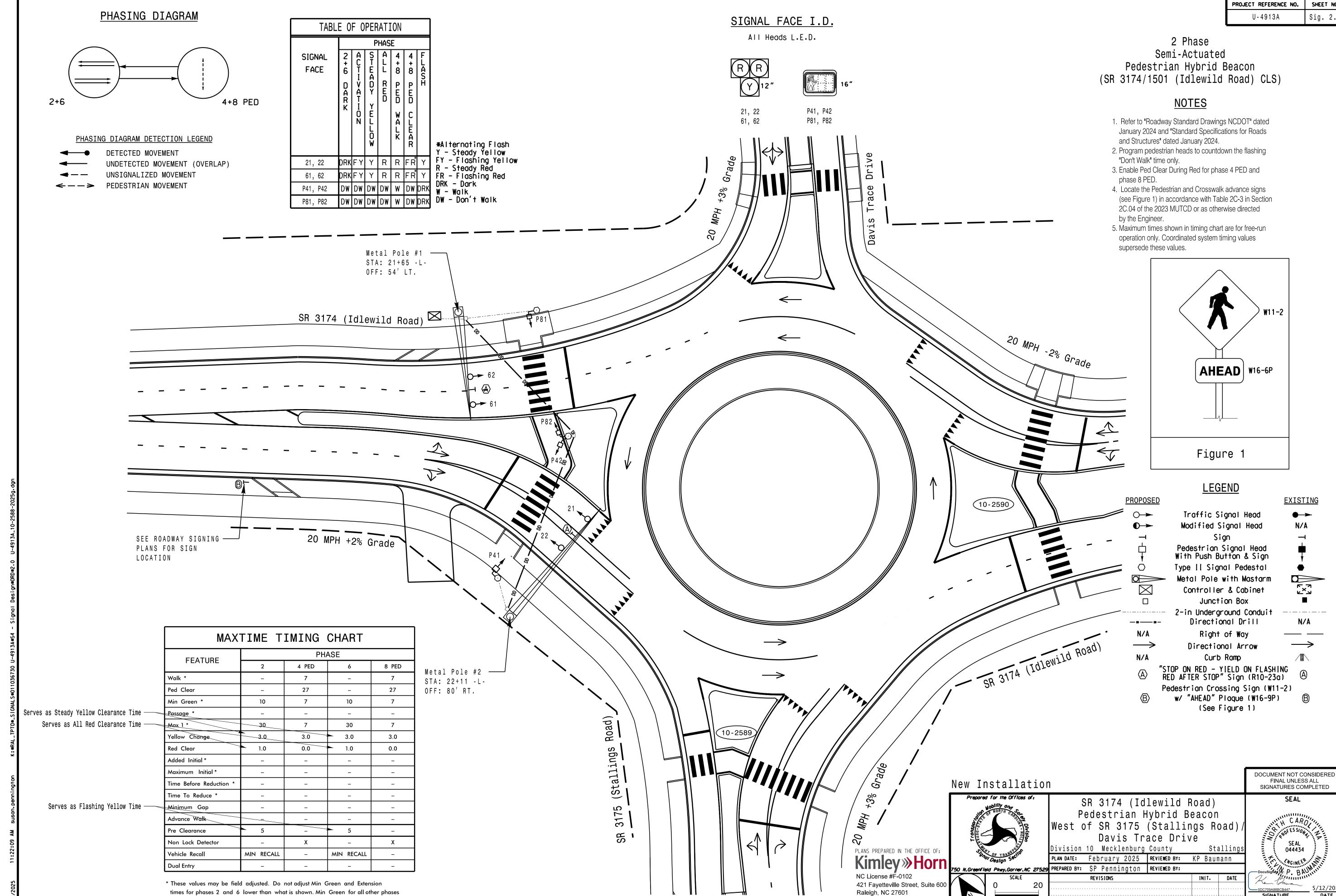
times for phases 2 and 6 lower than what is shown. Min Green for all other phases should not be lower than 4 seconds.
