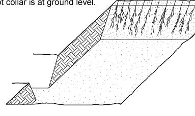
5. Place a 2 inch layer of well rotted sawdust over the roots maintaining a sloping angle.
