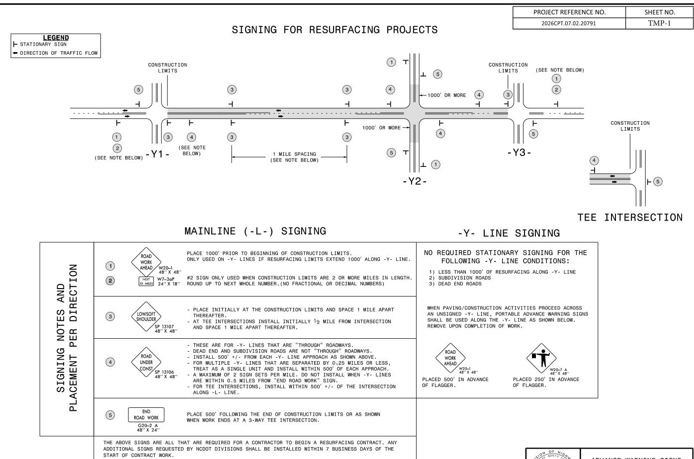
FOR RESURFACING MAPS WITH CONSTRUCTION LIMITS LESS THAN 2 MILES IN LENGTH, NO STATIONARY SIGNS ARE
