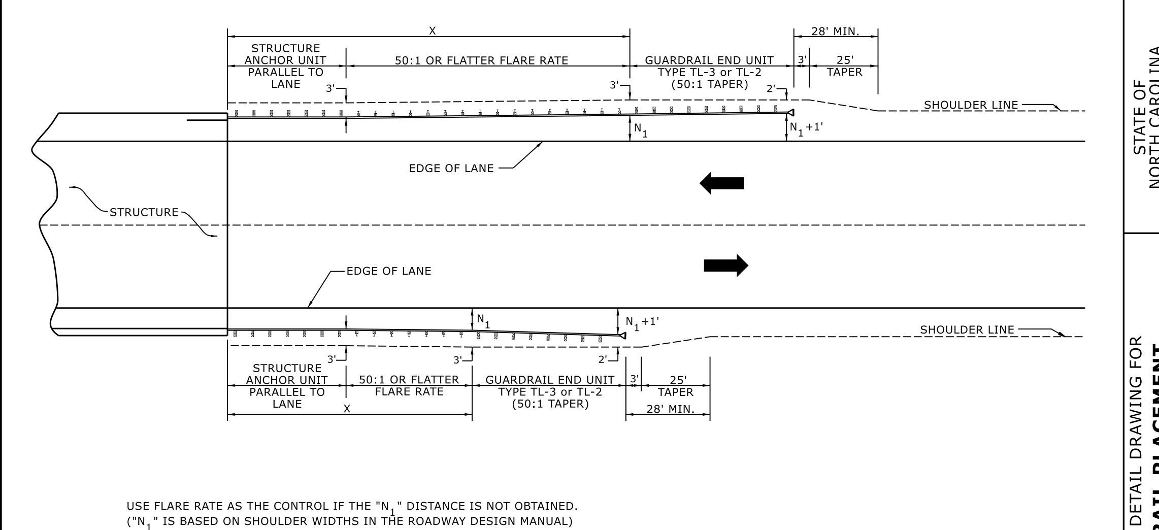
LENGTHS AND OFFSETS FOR PROPOSED GUARDRAIL AT TWO LANE - TWO WAY LOCATIONS
