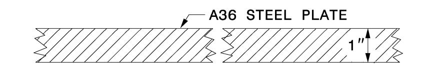
SECTION VIEW OF STEEL TOP PLATE
