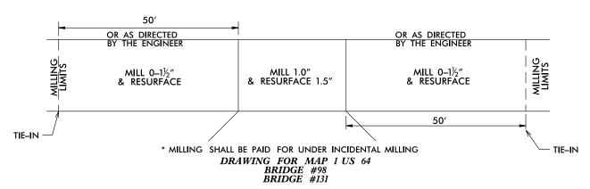
NOTE: DO NOT FILL IN DRAIN HOLES DURING RESURFACING.
