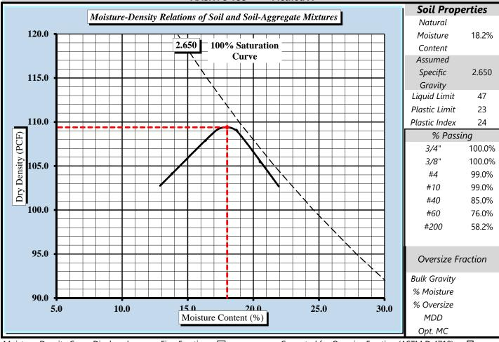
Moisture-Density Curve Displayed: Fine Fraction 🗵 Corrected for Oversize Fraction (ASTM D 4718) Sieve Size used to separate the Oversize Fraction: #4 Sieve 区 3/8 inch Sieve 3/4 inch Sieve Mechanical Rammer Manual Rammer ⊠ Moist Preparation □ Dry Preparation 区 ND=Not Determined. References / Comments / Deviations:
