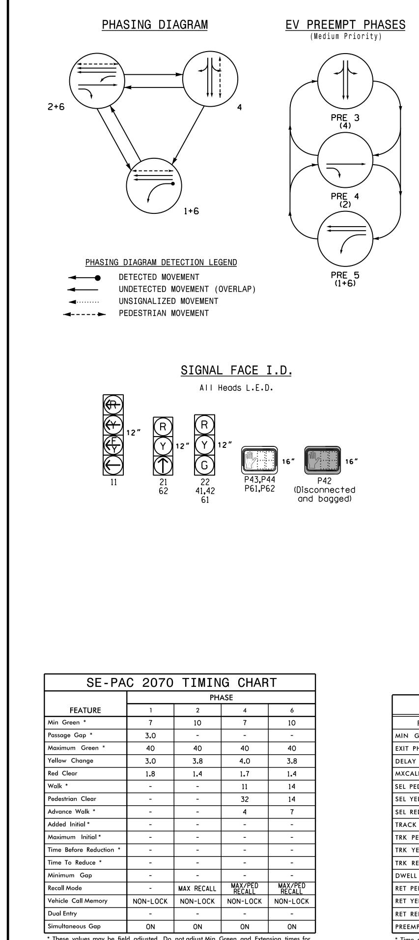
\* These values may be field adjusted. Do not adjust Min Green and Extension times for phases 2 and 6 lower than what is shown. Min Green for all other phases should not be lower than 4 seconds.
