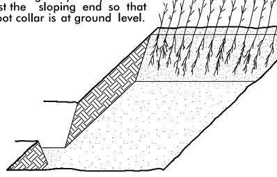
5. Place a 2 inch layer of well rotted sawdust over the roots maintaining y // a sloping angle.
