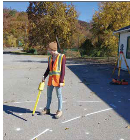
Photo 2. Checking magnetic anomalies with the Schonstedt to mark the perimeter.
