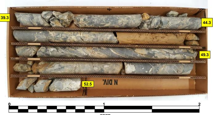
**GEOLOGICAL STRENGTH INDEX: GSI** 39.3' - 47.4' : 15 - 25 \*CLAY IN-FILL 46.3'-47.3' 47.4' - 52.5' : 30 - 40
