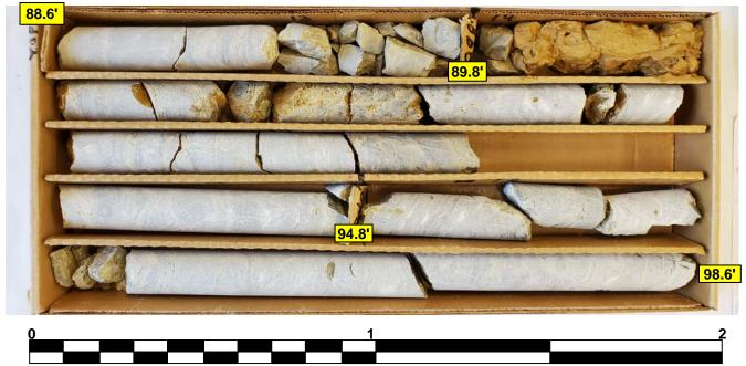
**GEOLOGICAL STRENGTH INDEX: GSI** 88.6' - 90.9' : 15-20 \*w/ CLAY IN-FILL ZONES 90.9' - 98.6' : 30-40
