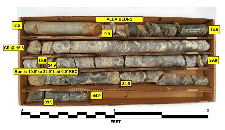
**GEOLOGICAL STRENGTH INDEX: GSI** 16.8' - 19.9' : 30 - 40 19.9' - 24.9' : Barrel had NO RECOVERY 24.9' - 44.9' : 10 - 15
