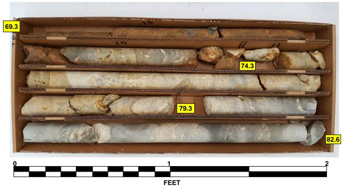
**GEOLOGICAL STRENGTH INDEX: GSI** 69.3' - 75.0' : 10 - 20 \*N.C.R. w/ CLAY IN-FILL ZONES 75.0' - 82.6' : 40 - 50
