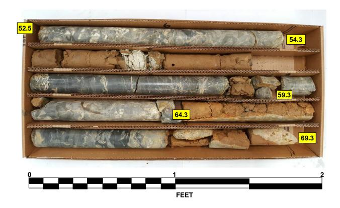
**GEOLOGICAL STRENGTH INDEX: GSI** 52.5' - 54.3' : 45 - 55 54.3' - 69.3' : 15 - 25\* \*N.C.R. w/ CLAY IN-FILL ZONES
