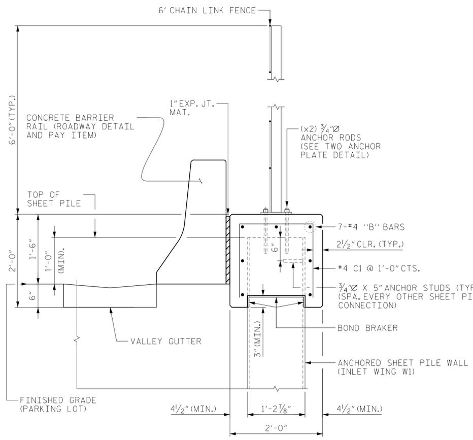
CONCRETE BULKHEAD AND CHAIN LINK FENCE DETAIL
