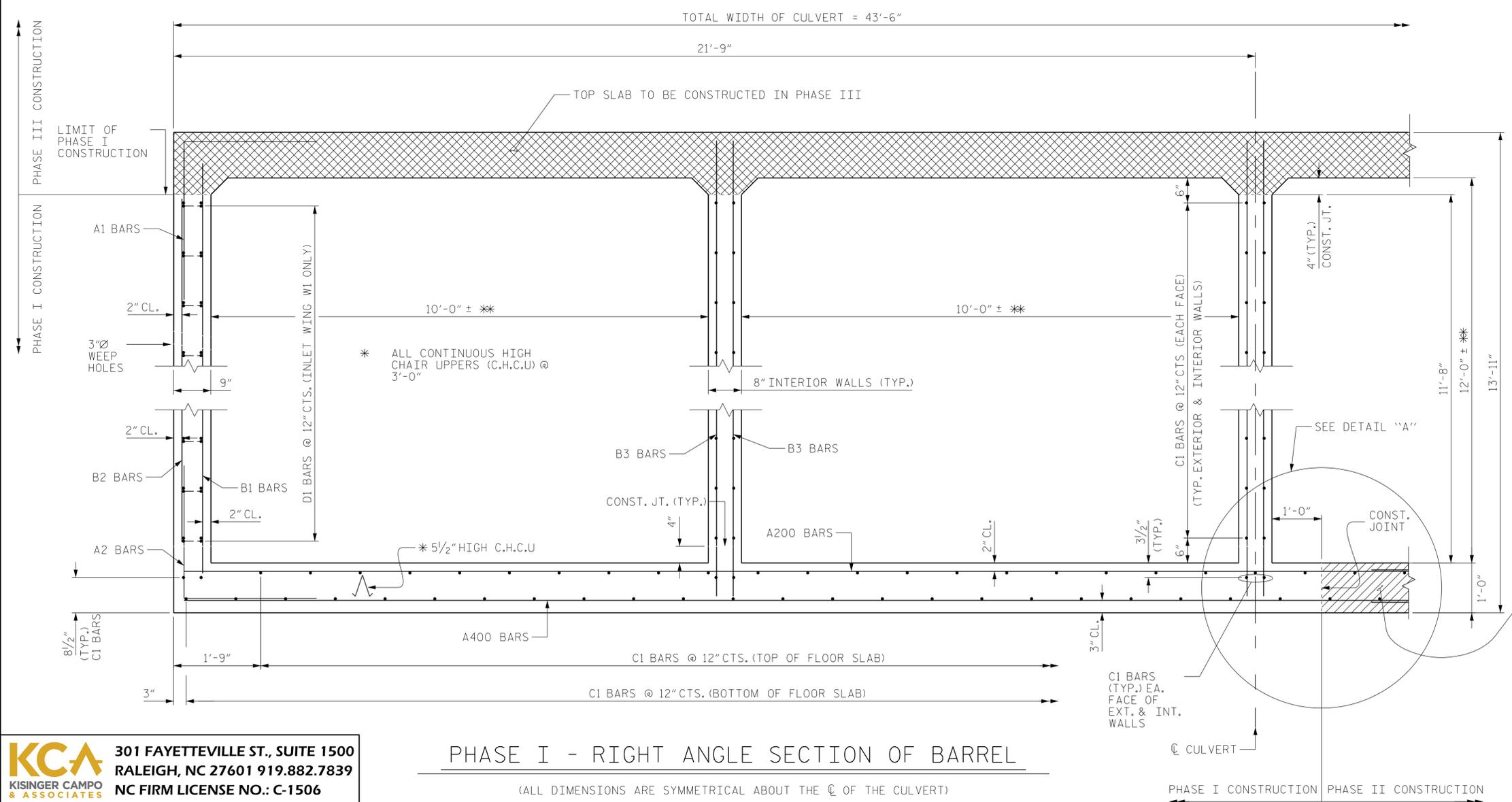
PHASE I - RIGHT ANGLE SECTION OF BARREL
