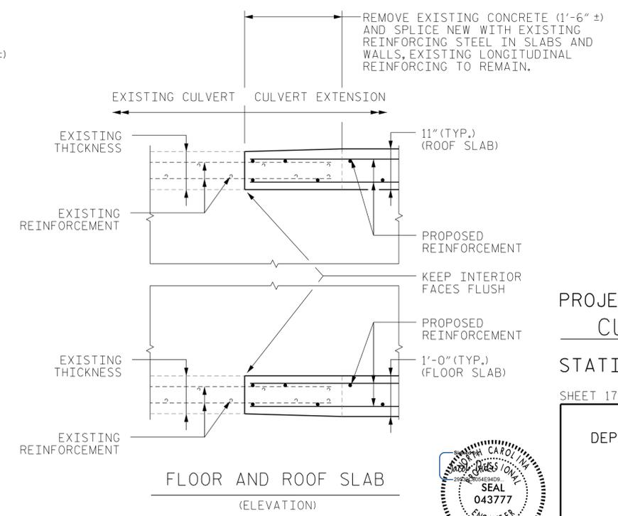
FLOOR AND ROOF SLAB
