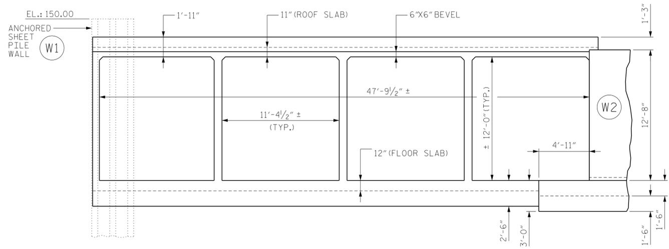
END INLET ELEVATION NORMAL TO SKEW
