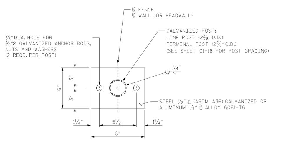
TOP VIEW - TWO ANCHOR PLATE DETAIL
