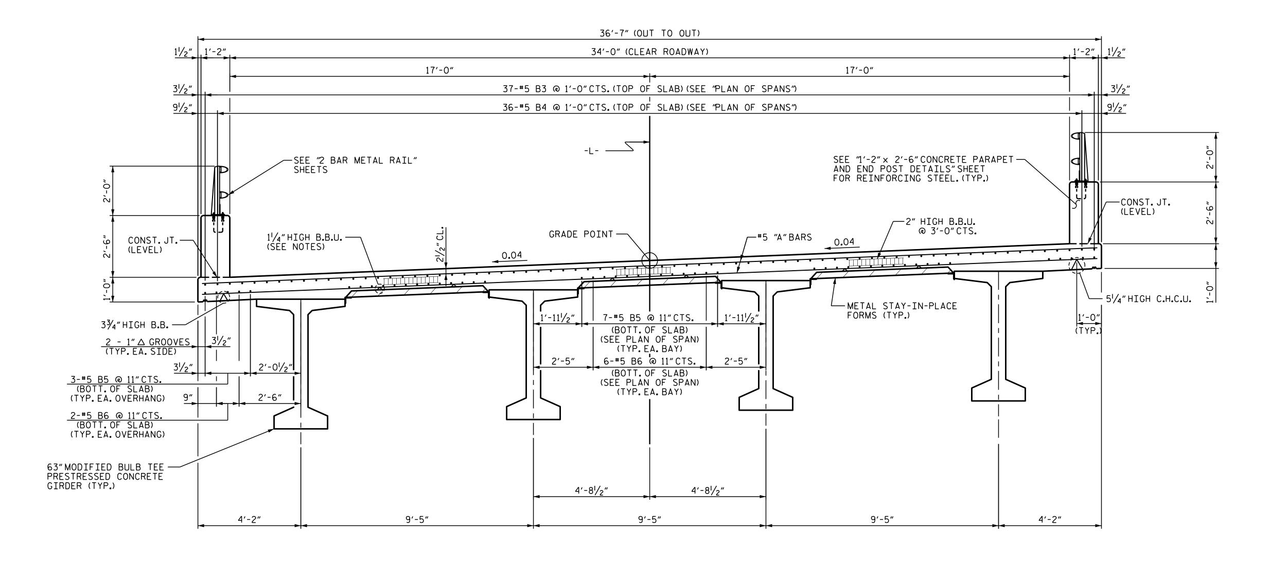
TYPICAL SECTION AT LINK SLAB AT BENT
