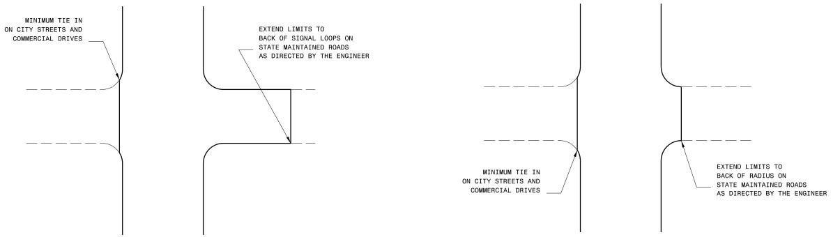
TYPICAL DETAIL OF PROJECT LIMITS AT SIGNALIZED Y LINES
