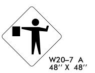
PLACED 500' IN ADVANCE OF FLAGGER. PLACED 250' IN ADVANCE OF FLAGGER.
